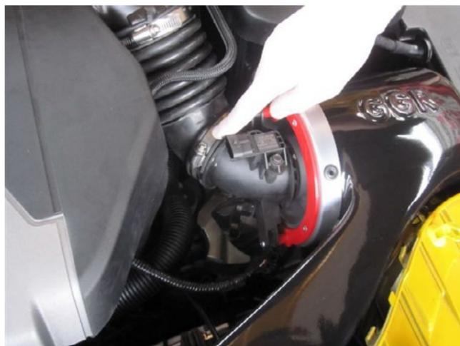
16. Refit the airflow sensor plug. release cable.
