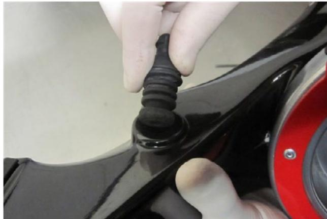
14. Refit GGR CAIS carefully onto the front air intake and then into its mounts.
