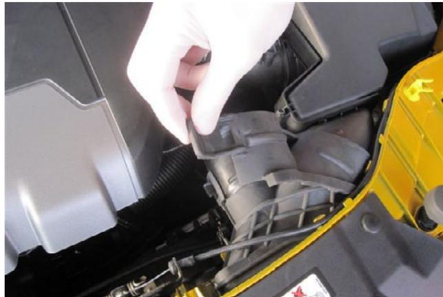
4. Carefully lift the airbox up and out of its rubber mounts.
