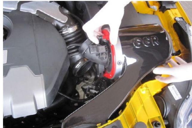
15. Refit and tighten the air intake hose clip.
