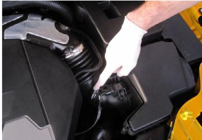
2. Carefully disconnect the airflow sensor.
