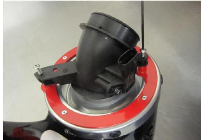
13. Refit the rubber bobbin into the GGR CAIS using a small amount of lubrication.
