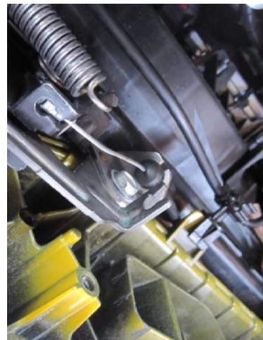
9. Remove intake elbow from standard airbox.
