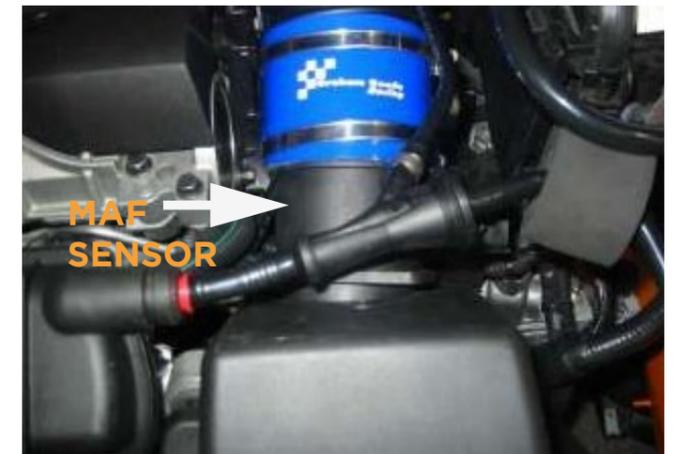
**7** Carefully remove the original air box assembly. This sits in the engine compartment on 4 pegs in the base of the unit, which press into 4 corresponding rubber bushes. Carefully pull the air filter upwards to disengage the pegs from the bushes (the pegs are approximately 25mm long). Once the air filter assembly is loose, it can be removed by first slightly lifting the right-hand-side whilst sliding the assembly also to the right, then lifting it free from the engine.
