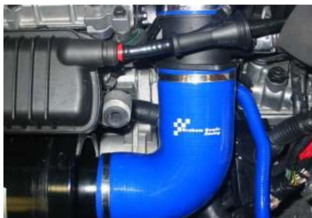
**18** Re-secure the air inlet duct using the original fixings, check and adjust the alignment of the hoses, tighten all of the hose clips and refit the black plastic slam panel cover.
