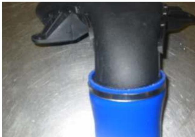
**17** Fit the MAF sensor inlet to the 'long' end of the large silicone 90° elbow, the short silicone hose to the MAF sensor outlet, then connect the elbow to the CAIS outlet, and the short hose to the turbo cross-pipe as shown. Do not tighten any hose clips at this point.
