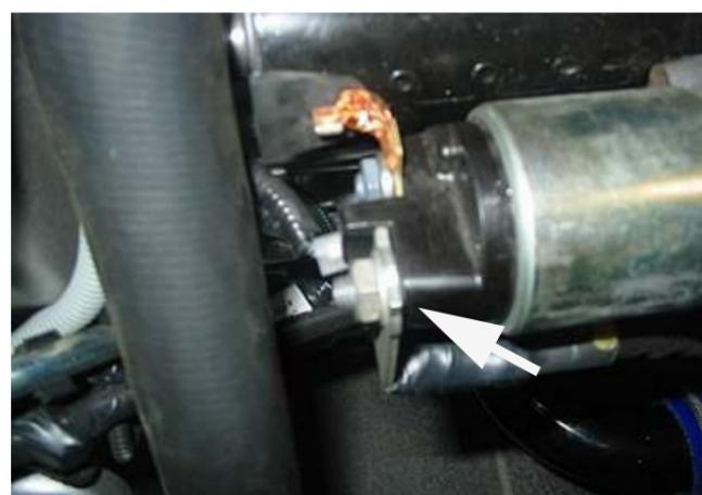
**10** Glue the small piece of black foam supplied to the breather system tank as shown.
