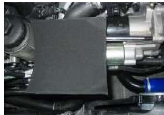
**13** The new CAIS can now be slid into place onto the mounting saddle as shown. clearance.
