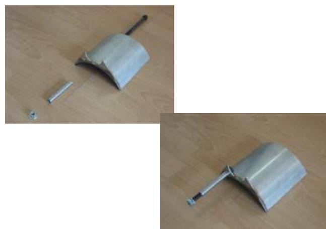
**12** Pass the threaded section of the bolt through the hole vacated by the dowel and tighten into position using the nut provided. (The circular cut-out in the saddle bracket is shaped to locate the assembly in the correct position, to prevent any misalignment issues. Just make sure that the bracket seats correctly).
