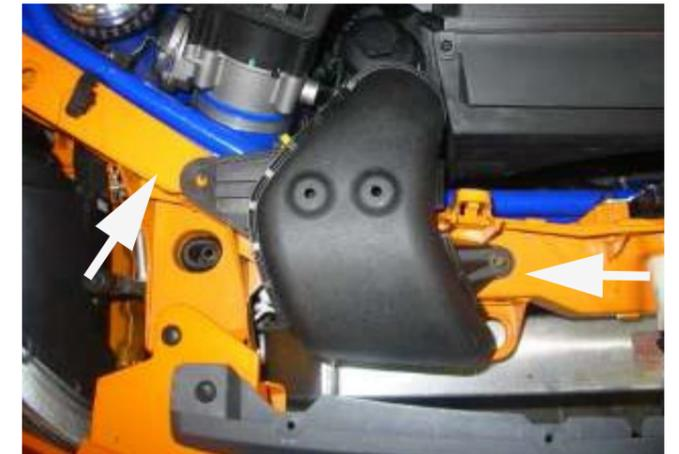
**6** Remove the short hose connecting the Mass Air Flow sensor to the cross-pipe, and then remove the two Torx headed screws holding the MAF sensor to the airbox. Put the MAF sensor carefully to one side.
