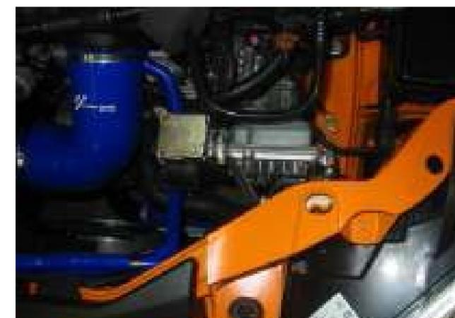
**22** From underneath the car, carefully raise the coolant radiator back into its original position and secure in place with the cradle and screws removed in step 2.
