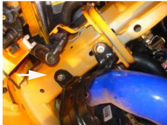
**3** On top of the car now, remove the 4 Torx screws that retain the ECU to the airbox, and move the ECU to one side.
