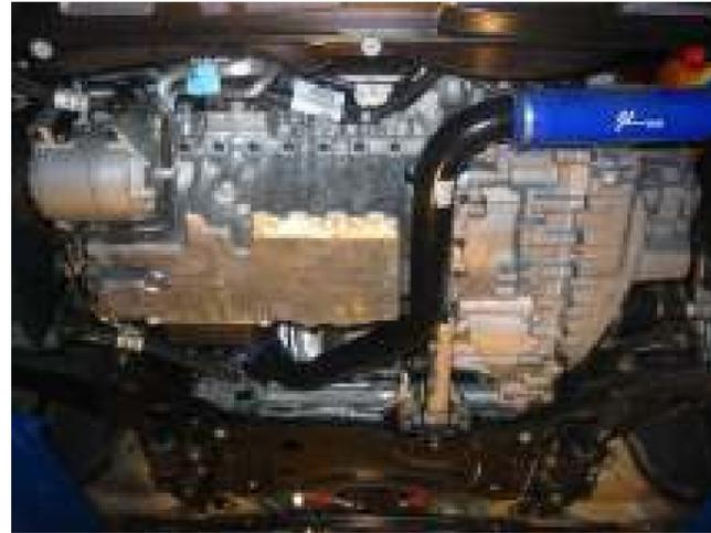
**2** Remove the two radiator support cradle screws in the front of the chassis legs, and carefully lower the radiator.
