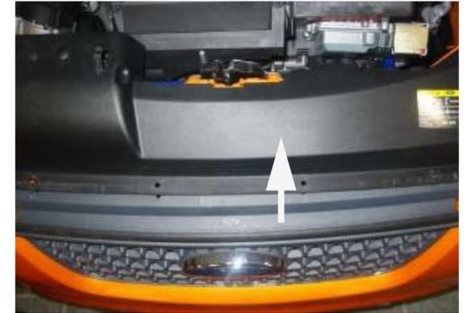
**5** Remove the air inlet duct retainers from the bonnet slam panel, and lift the duct away from the airbox.
