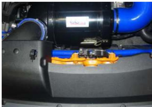
**19** To secure the CAIS in place the large hose clips supplied have to pass around the filter body and the mounting saddle at each end as shown. We suggest that the retaining screws are positioned below the filter, on the retaining saddle, to prevent damage to the softer aluminium filter body. Do not over-tighten these clips, as they are only to hold the filter in place!
