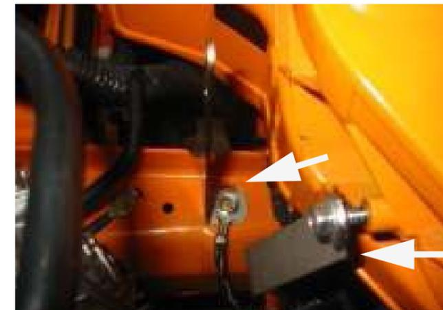
**21** The ECU can now be fixed in place using the three M6 nuts and bolts supplied. The ECU unit is completely sealed, and there should be no problems with mounting it in this new position.
