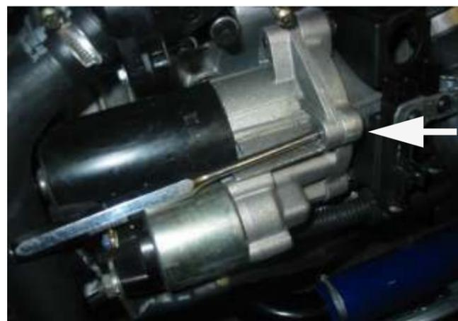
**9** Loosen the retaining nut, and rotate the starter solenoid power lead (if required) as shown, to give additional clearance.
