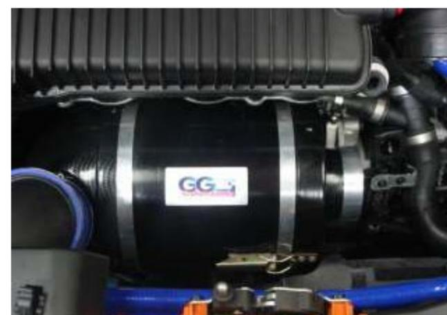
**14** Carefully cut the top ring (as shown) from the air intake pipe and re-fit this to the air inlet duct.
