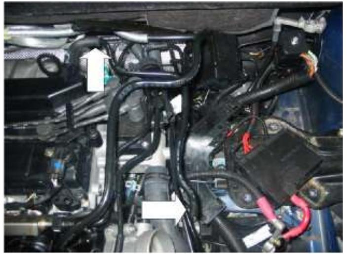
Loosely assemble the silicone hose onto the CAIS (pushing the hose onto the CAIS, then onto the throttle inlet, and push the breather hose into the stub on the inlet hose) and fit into position:
