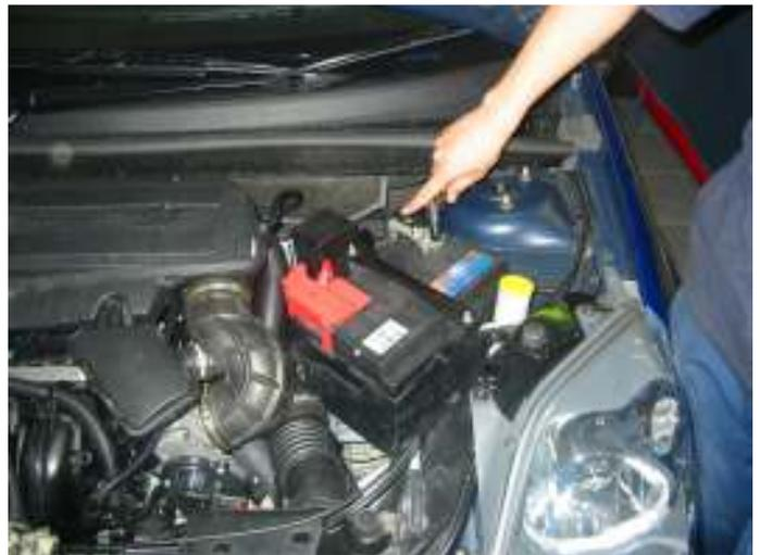
Remove the battery and then the battery box:
