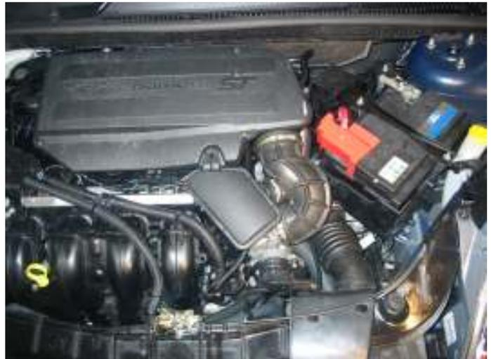
Disconnect both battery terminals and the retaining clamp: **Make sure that you know your radio security code before disconnecting the battery.**
