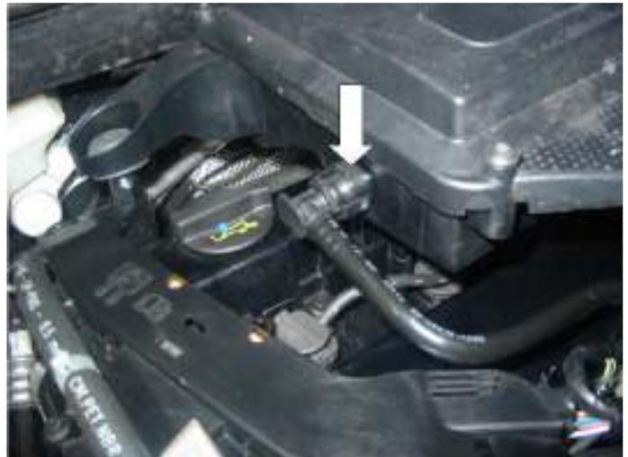
Carefully lift the standard airbox up out of the three rubber mountings on the top of the engine, making sure that all hoses are free and un-clipped.
