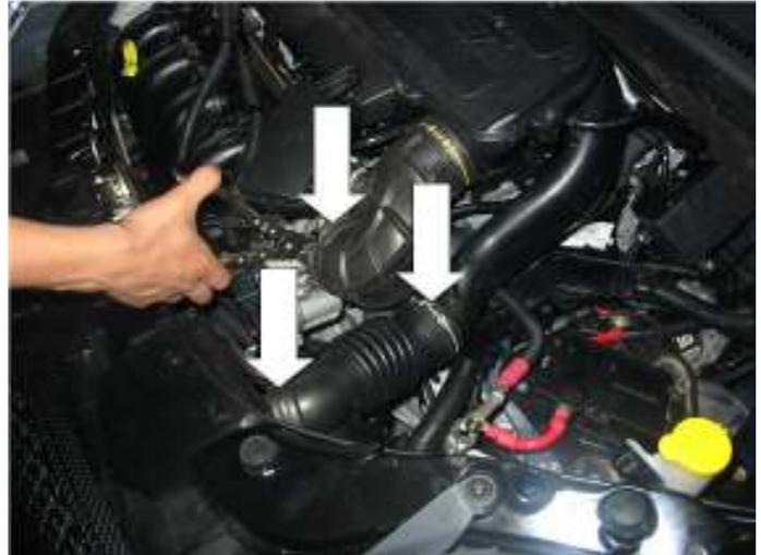
Press the sides of the clip to enable you to remove the breather pipe from the standard airbox:
