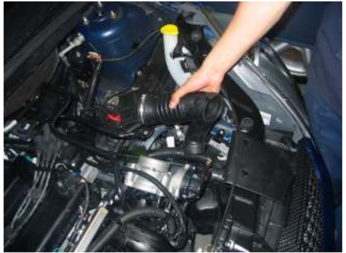
Un-screw the two screws in the bonnet slam panel retaining the air inlet scoop and remove the scoop:
