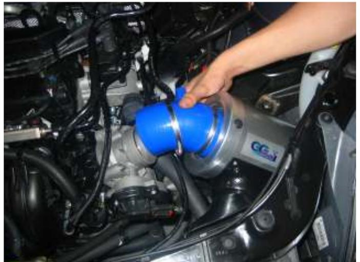
Fit the stainless steel mounting bracket as shown between the CAIS base and the ECU mounting plate bracket upper bolt.
