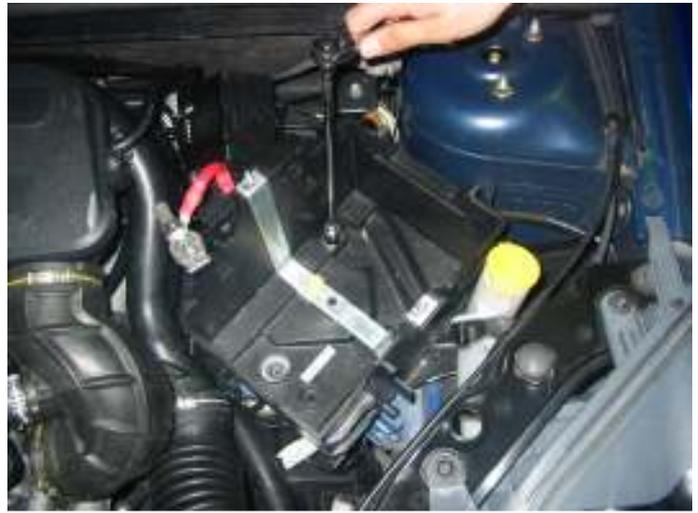
Remove these three hose clips. One from the airbox to throttle body hose, and one from each end of the resonator hose:
