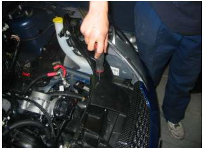
Pull the resonator chamber up out of its three rubber mountings, then remove this from below the engine compartment:
