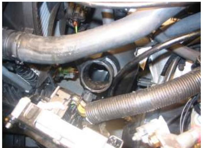
Cut the original breather system pipe as shown, ready for re-fitting to the new inlet hose (the section to be use is shown arrowed):
